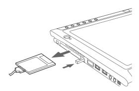
Figure 2-6. Removing a PC Card
